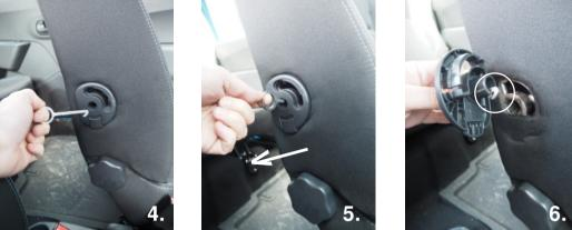
Remove the plastic cover panel by placing the enclosed «key-hook tool» in the center hole. Make sure that the hook tool is grabbing the lower front hook on the cover panel (see pict.6). Then pull straight outwards until the plastic cover panel is released!
