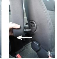
Remove the original armrest by pushing the lock-sprint on the plastic cover panel -then fold down the armrest and pull it outwards until it is released.
