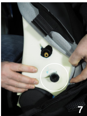
(7) Fold back the foamrubber over the adapter bracket, to it's original position, and cut a hole for the adapter tube. Then restore the upholstery!!!
