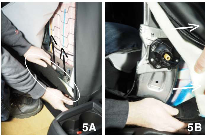
(5A) Release the "back-curtain" by pulling it straight upwards (5B) then push the foamrubber forward and away over the side of the seat -until you see the frame.
