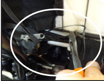
...and cut the cable-tie that secures the zipper handle under the seat.
