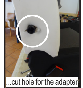
Fold back foamrubber in the original position... ...cut hole for the adapter
