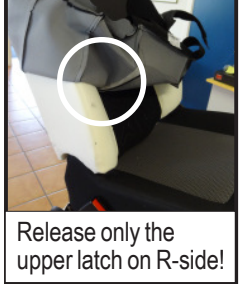
Release only the upper latch on R-side!
