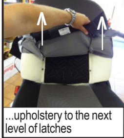
Continue to pull up the... ...upholstery to the next level of latches
